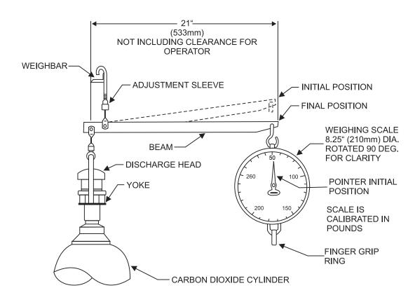
TO WEIGH CYLINDERS: REMOVE CONTROL HEAD, IF USED. LOOSEN CYLINDER FROM FRAMING. HANG HOOK ON WEIGHBAR. PLACE YOKE UNDER DISCHARGE HEAD. USE ADJUSTMENT SLEEVE TO BRING BEAM TO INITIAL POSITION. PULL DOWN ON FINGER GRIP RING UNTIL BEAM IS IN FINAL POSITION. READ WEIGHT ON WEIGHING SCALE. DEDUCT 3.75 LBS. FOR DISCHARGE HEAD ALLOWANCE. RESULT IS WEIGHT OF CYLINDER.
